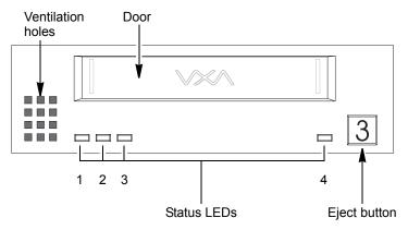
Figure 3-1 Internal tape drive: front-panel components
